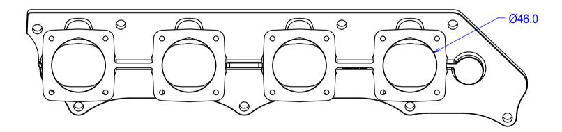
Flanges for Jenvey SF throttle bodies. May be ported out to 52mm at body flange and proportionally at head flange. Undrilled bosses on top side for injector ports, vacuum tappings etc.
